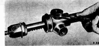
Fig. 18. Using feeler gauge to determine shim thickness required under cap nut
